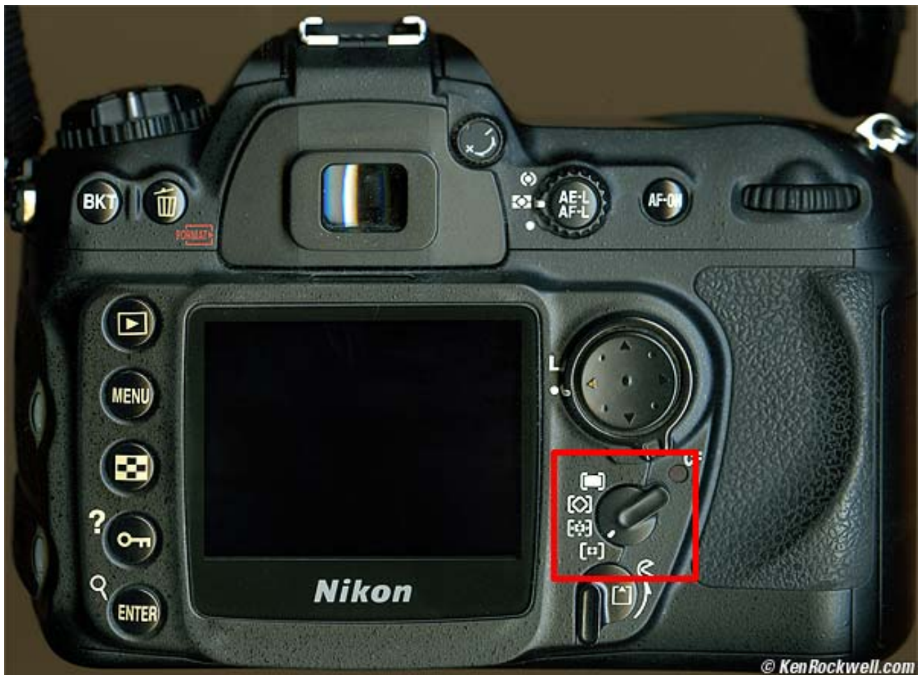
D200 AF Area Mode Switch. Here it's set to use a single AF area.
